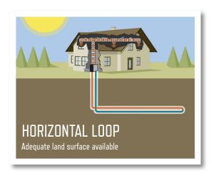
Horizontal loops use 100-350 feet long pipes placed in trenches below the frost line. The majority of horizontal installations in lowa use a slinky coil loop. This design allows three times the amount of pipe to be installed (laid upright or flat) in a trench.
