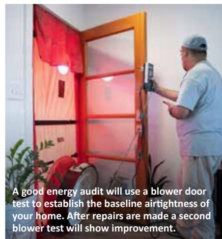
A good energy audit will use a blower door test to establish the baseline airtightness of your home. After repairs are made a second blower test will show improvement.
